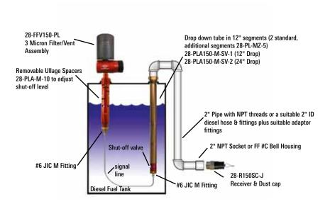
A std 28-PLA150-M-SV-7 that has a 7" segment is available for shallow pontoon diesel tanks and top fill
