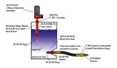
**Internal Signal Line for Remote Fill Pressureless Diesel Tanks** Kit P/N 28-PLA150-MARFFVDM
