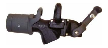
The Titan nozzle is the smallest and lightest diesel nozzle industry wide with an all metal housing, a non-slip powder-coated finish and has the most forgiving latching mechanism in dirty conditions. The unique patent pending design allows the nozzle to be field repairable. The one piece replacement cartridge means that field repair only involves removing the handle and replacing the cartridge.
