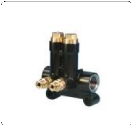
Piston distributor, group VKS02 0.1 to 0.4 cm 3 metering with universal quick connectors
