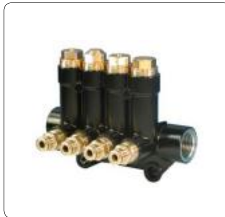
Piston distributor, group VKS04 0.1 to 0.4 cm 3 metering with universal quick connectors
